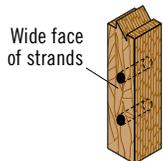
In order to use the manufacturer's published capacities when designing column caps, bases, or holdowns for uplift, the bolts or screws must be installed perpendicular to the wide face of strands as shown at left.
