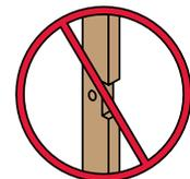
**DO NOT cut a notch and a hole in the same cross section**
