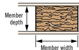
Some columns are listed in both beam and plank orientation. The first dimension is for member width, and the second dimension is for member depth (wall thickness).
