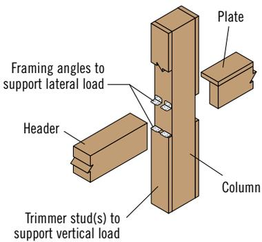
**L13** Plate width must equal the wall thickness to provide lateral bracing. (Plate not required if header width equals the wall thickness.)
