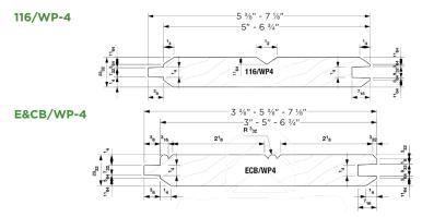
Above are Interfor's two most commonly run profiles diagrammed in 1x6.
