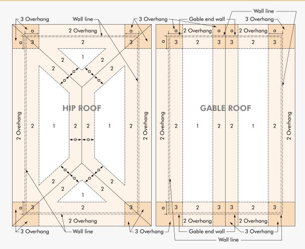
Distance a = 4 ft in most cases (10% of least building width or 0.4 times building height, whichever is smaller, but not less than either 4% of least building width or 3 ft).
