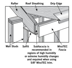
\* Note: Nail at least 1/2" from the edge. Do not nail into the edges of MiraTEC trim. For 4/4 and 5/4 fascia and soffit applications, MiraTEC trim can be fastened directly to the rafter ends, double nailed a maximum of 24" on center. For 5/8 fascia and soffit applications, MiraTEC trim must have a sub-fascia and be nailed 16" on center to the rafter ends or sub-fascia. For all other horizontal and vertical applications, double nail 16" on center, falling on the studs.
