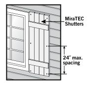
MiraTEC trim can be used to make decorative shutters. The shutter must be fastened to the home a minimum of 24" on center around the perimeter of the shutter as shown in the illustration. Working shutters will not be covered by the MiraTEC limited warranty based on the inability of providing adequate fastening on the non-hinge side of the shutter.
