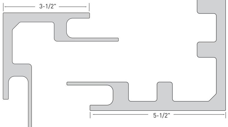
**Kleer Konceal** has a built-in 3/4" reveal that covers rough cuts at corners and other areas where precision cuts are time consuming and difficult. Meaning you save time without sacrificing that striking, finished look. Suitable for use with vinyl, fiber cement or wood siding, Kleer Konceal is available in smooth or natural woodgrain textures that ensure appealing aesthetics and lasting value.
