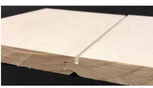
**Primed Radiata T&G Nickel Gap**, often called Shiplap, is a pre-primed interior wall paneling. It is a tongue and groove product with a self-spacing 1/8" nickel gap reveal. This is a finger jointed product made of clear Radiata Pine blocks that are knot and void free. It is finished with two coats of an acrylic latex primer and the face is buffed for a smooth finish that is ready to paint immediately.
