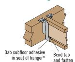
Seat the joist tight to the bottom of the hanger. When using hangers with tabs, bend the flange tabs over and nail to the TJI® joist bottom flange. Placing a dab of sublfoor adhesive\* in the seat of the hanger prior to installing the joist can reduce squeaks.
