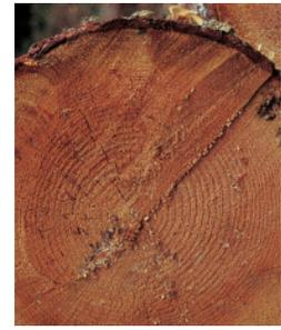
Douglas Fir sapwood is white to pale yellow while the heartwood is russet or orange-red; the timber often has a slight rosy cast with distinct growth rings. When freshly milled, timber has a characteristic resinous odor.
