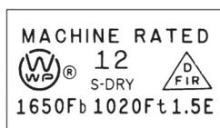
The grade stamp on MSR lumber indicates the machine stress-rating system used meets requirements of the grading agency's certification and quality control procedures. The grade stamp includes the phrase "Machine Rated" along with the E and  $F_b$  ratings. The stamp will also include the allowable tensile stress parallel-to-grain ( $F_t$ ),
