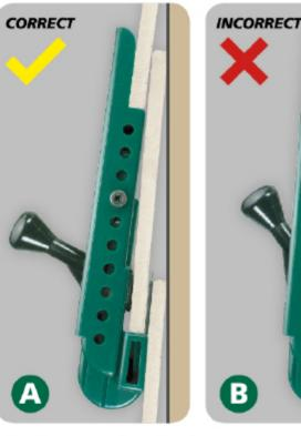
NOTE: Over-tightening handle may cause tool to pull away from siding. As the rubber pad naturally wears over time, the handle can be engaged further for continued use.
