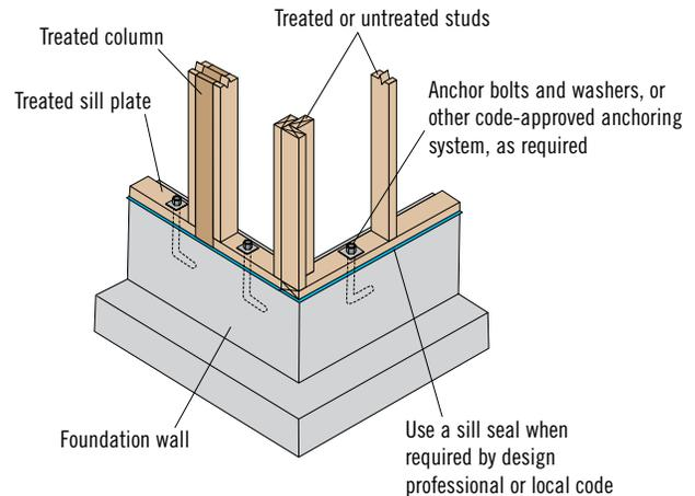
*StrandGuard® TimberStrand® LSL framing materials are intended for use in aboveground, protected applications such as sill plates, columns, and studs. The American Wood Protection Association (AWPA) standards classify such applications as Use Category 2.*
