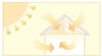
Radiant energy transferred through standard roof sheathing creates heat build-up in the attic. With no barrier to restrict the heat, it radiates through the insulation into living spaces, causing room temperatures to rise. More energy is needed to cool the house, and that means higher energy costs for homeowners.
